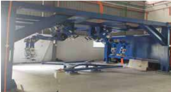
Headlining Yaskawa Robot Arm Cutting Process
